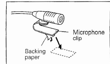
2 Adjust the horizontal orientation of the microphone in such a way that it faces towards the driver.
